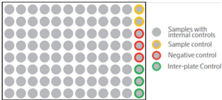
Figure 2. Plate layout for Olink Target 96 analysis. Column 12 contains pooled plasma controls (provided by the Discovery Proteome Center) as well as negative controls and plate controls (provided with the Olink kit).
